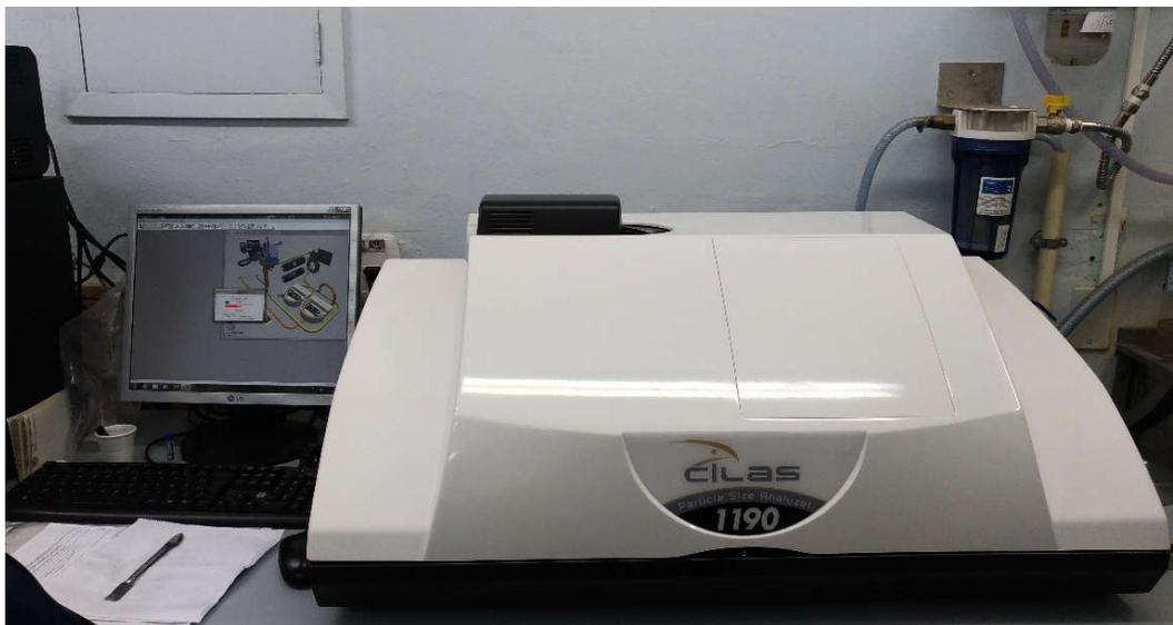
Figura 5: Cilas Particle Size Analyzer 1190
